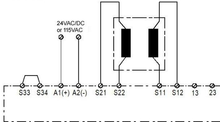
**Figure 7: Dual-Channel (With Wire-Break Safety) Configuration**
