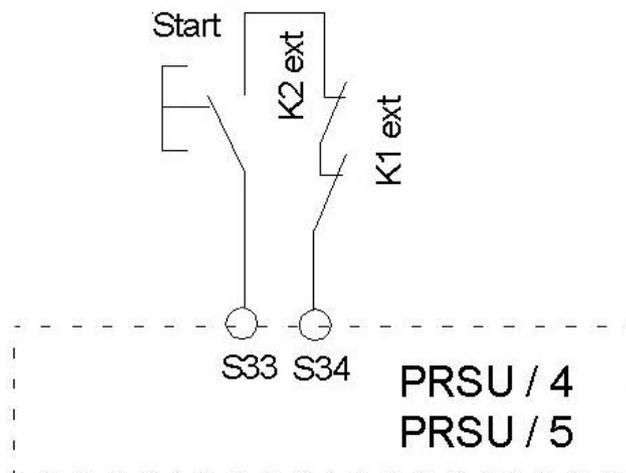
**Figure 6: RESET Mode (Conditional) Configuration**
