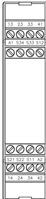
**Figure 2: Screw Terminal Numbering (Device Front Face)**
