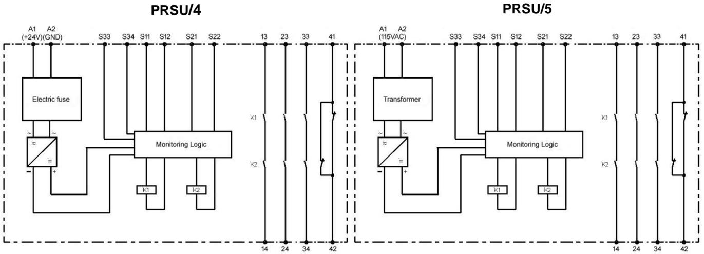
**Figure 1: Functional Schematics**
