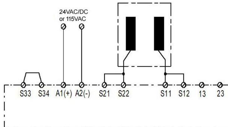
**Figure 8: Single-Channel (Non-Safety) Configuration**
