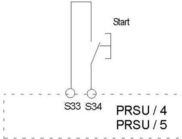
**Figure 5: RESET Mode (Manual) Configuration**
